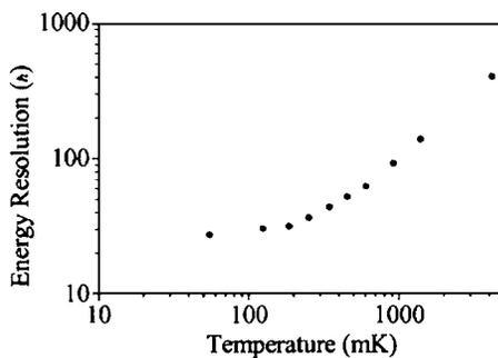
FIG. 4. SQUID energy resolution in number of quanta at 11 654 Hz as a function of temperature.
