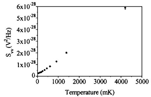
FIG. 2. SQUID noise spectral density  $S_{vv}$  at 11655 Hz as a function of temperature.
