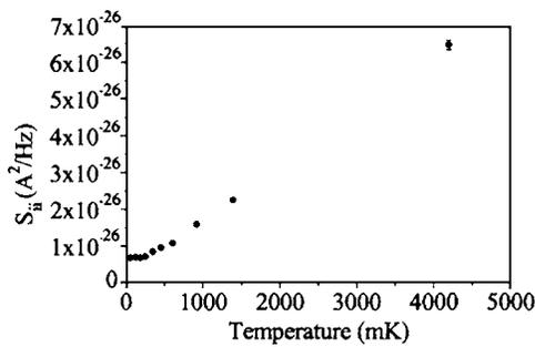
FIG. 3. SQUID noise spectral density  $S_{ii}$  in the frequency range of 10–11 kHz as a function of temperature.
