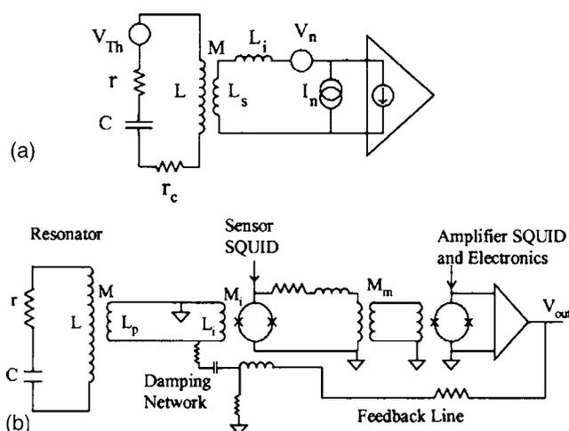
FIG. 1. (a) The noise model of the resonator-SQUID system. The two-stage SQUID is modeled by an ideal current amplifier with the noise sources  $V_n$  (back action noise) and  $I_n$  (additive noise). (b) Schematic circuit diagram of the resonator-SQUID system. The flux gain between the first and second SQUID is adjusted by means of the superconducting transformer  $M_m$ .
