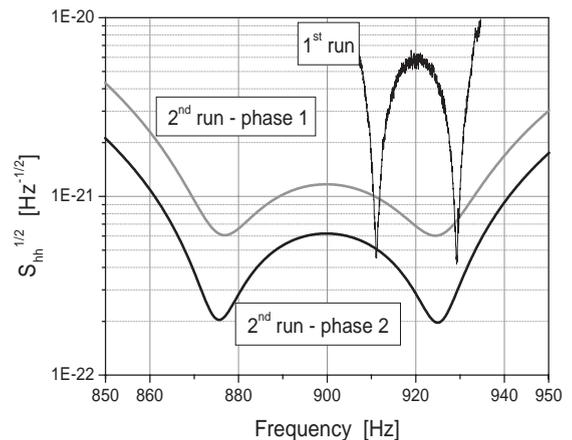
Fig. 1. Expected sensitivity for the next run of AURIGA: the first phase (gray thick line) will be at cryogenic temperatures ( $\sim 1$  K) while the second phase (black thick line) at ultracryogenic temperatures ( $\sim 0.1$  K). For comparison we also show the experimental sensitivity obtained in the first run (thin black line).
