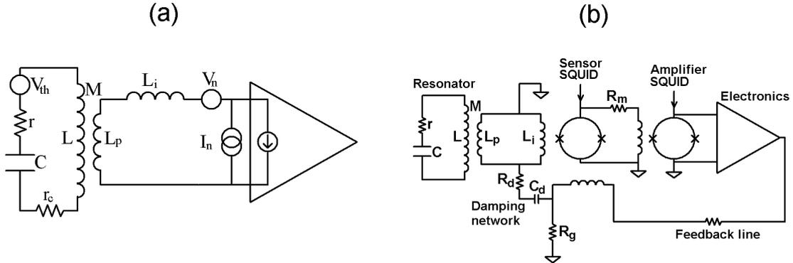
**Figure 1.** (a) Noise model of the SQUID coupled to the high  $Q$  electrical resonator. (b) Schematic circuit of the two-stage SQUID coupled to the high  $Q$  electrical resonator.
