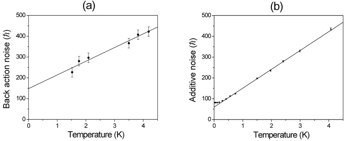
**Figure 2.** Measured power spectral densities of the SQUID noise sources, expressed in units of energy per unit bandwidth at  $\omega=\omega_0$ , as function of temperature: (a) back action voltage noise  $e_v=S_{vv}/(2\omega_0^2L_i)$  and (b) additive current noise  $e=S_{ii}\times(L_i/2)$ . Straight lines represent the linear fits of the experimental data.
