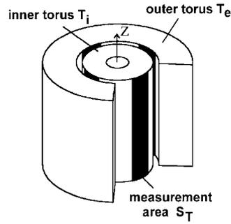
**Figure 1.** The detector is made of two concentric cylinders,  $T_e, T_i$ . The inner cylinder may also have null internal radius. The optimally oriented gravitational wave travels along the  $z$ -axis and induces relative displacements among the two cylinders. The output signal is obtained by measuring the relative distance in four regions (in black), each of area  $S_T$ , for the whole cylinder height.
