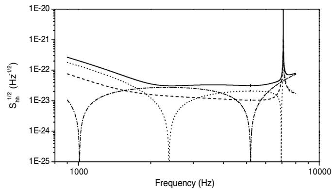
**Figure 2.** The contribution to the detector noise at the SQL is evaluated for a Mo detector. Continuous line: total noise. Dashed line: thermal noise evaluated at  $Q/T \sim 2 \times 10^{-7} \text{ K}^{-1}$ . Dashed-dotted line: amplifier displacement noise. Dotted line: amplifier back-action noise.
