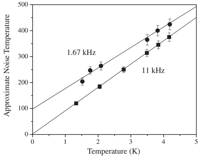
**Figure 2.** Approximate noise temperature of the two-stage SQUID amplifier expressed in equivalent number of quanta ( $k_B T'_n / \omega_0 \hbar$ ) as a function of the operation temperature at 1.67 kHz and at 11 kHz.
