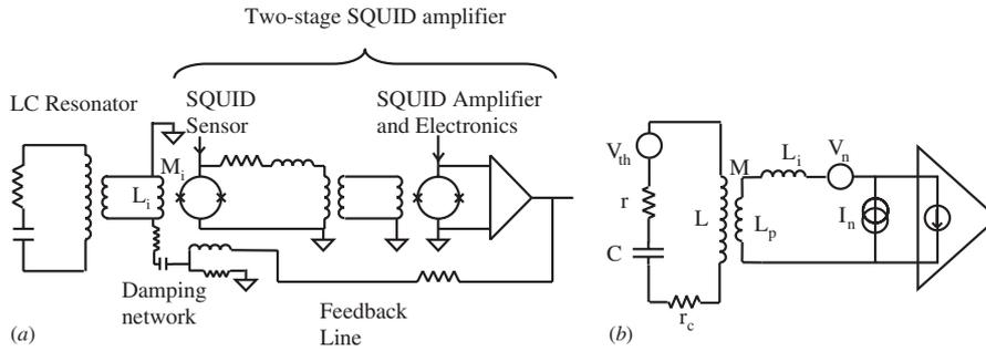
**Figure 1.** (a) Schematic circuit diagram of the two-stage SQUID coupled to the high- $Q$  LC resonator. (b) The noise model of the resonator-SQUID system. The two-stage SQUID is modelled by an ideal current amplifier with the noise sources  $V_n$  and  $I_n$ .
