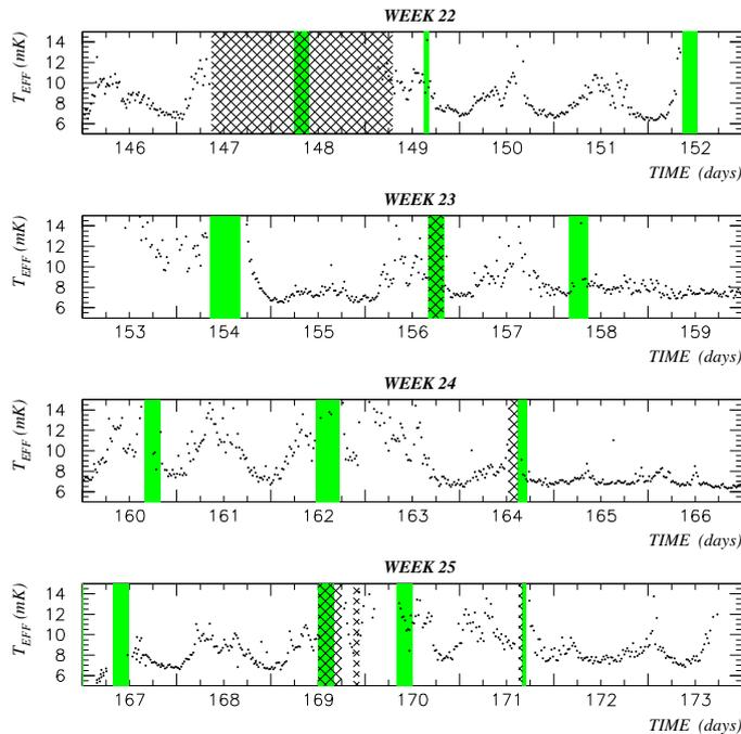
Figure 2: Noise temperature for bursts of the AURIGA detector for the first four weeks of full operation in 1997. Each point is a  $20 \text{ min}$  average. Noise temperature is below  $14 \text{ mK}$  for more than 70% of the time. Grey shades refer to 1 K pot refills, grids to calibration procedures .
