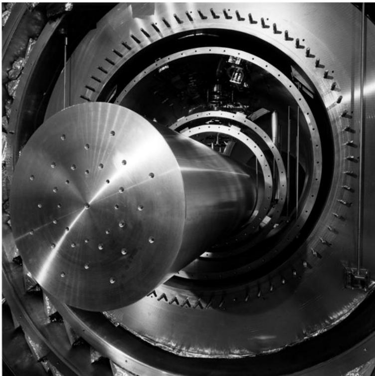
Figure 1: inner part of the AURIGA cryostat before the final assembly of the transducer and the thermal shields. It shows the bar, the inner stages of the suspensions made by ring-shaped masses and elastic rods, and the toroidal liquid Helium tank.
