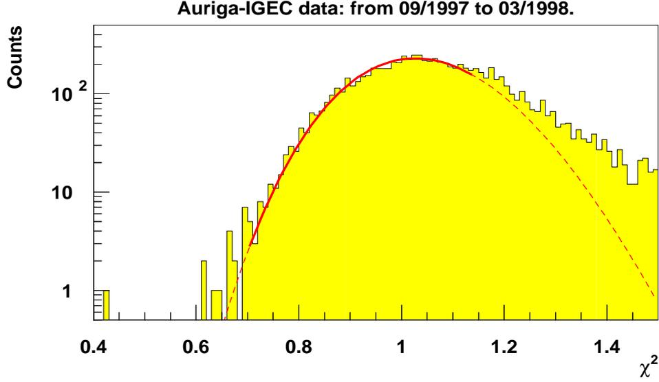
**FIGURE 5.** Histogram of the calculated  $\chi_e^2$  of the candidate events of the AURIGA detector under the IGEC Collaboration from Sept. 1997 to March 1998. These 15854 events have amplitude  $\text{SNR} > 5$  and are below a  $\chi_e^2$  threshold which corresponds to a false dismissal of about  $1 \times 10^{-4}$ . The  $\chi_r^2$  distribution is also shown as a continuous line.
