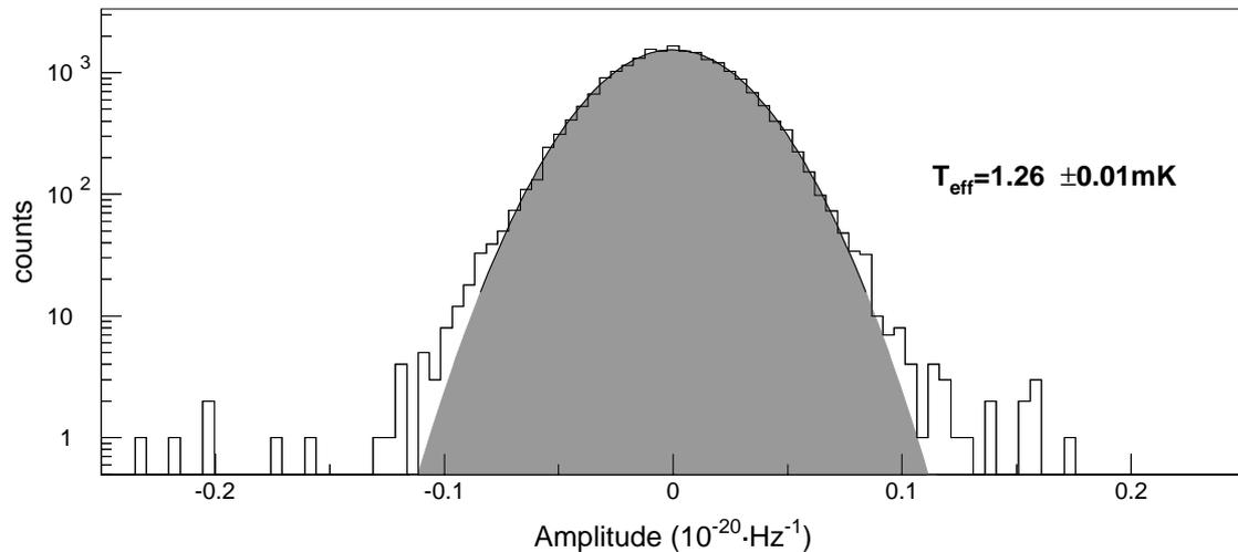
**FIGURE 4.** Amplitude histogram of filtered data during one day of satisfactory operation of the AURIGA detector. The data has been subsampled one per second to get almost independent samples. The small deviations from gaussian statistics at high amplitudes are due to the presence of signals overimposed on the noise.
