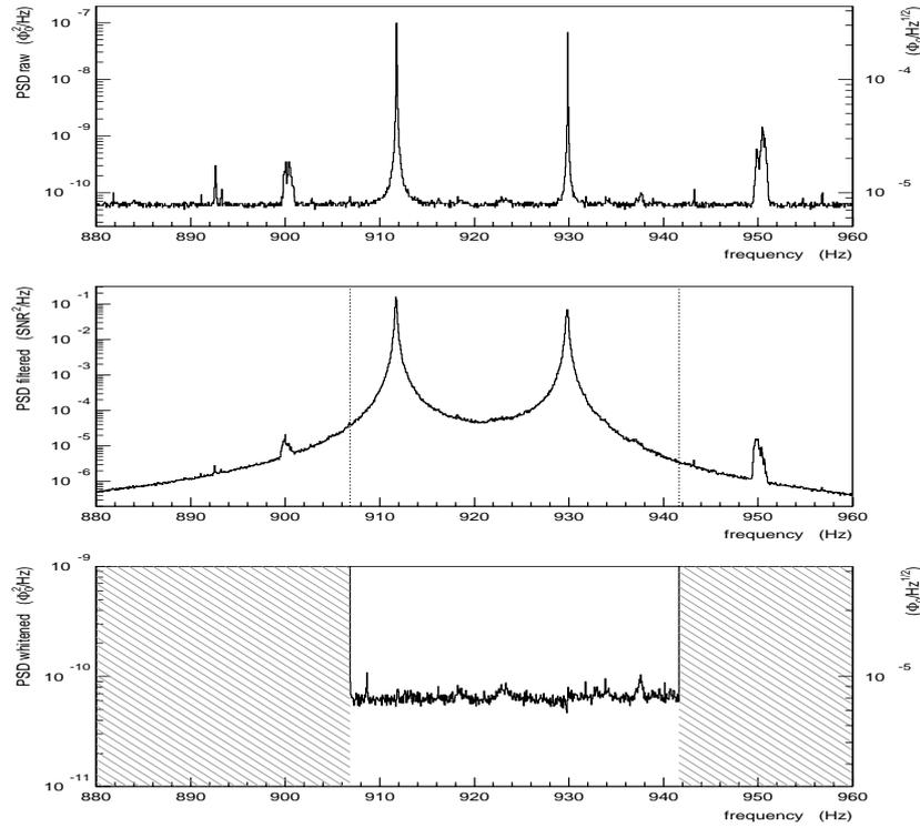
**FIGURE 2.** Noise power spectral density around the bar-transducer modes of AURIGA for: 1) raw data (upper); 2) W.K. filtered data (middle); 3) whitened decimated data (lower) for the same time period.
