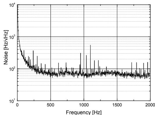
**FIGURE 2** Frequency noise of the free-running laser
