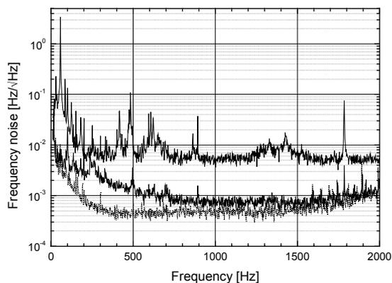
**FIGURE 3** Frequency noise for the laser locked to the reference cavity (upper curve); amplitude noise (middle curve); electronic noise (lower curve).
