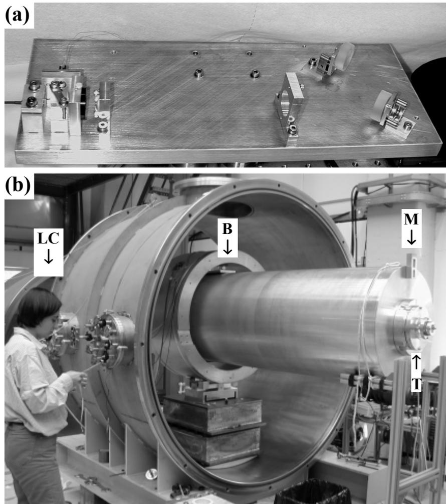
**FIGURE 7** (a) Close view of the optical bench. (b) Room temperature bar. LC: Livia Conti; B: optical bench; M: mirror; T: trasducer cavity.
