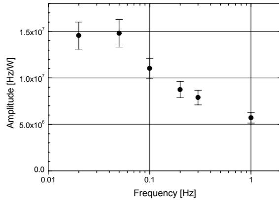
**FIGURE 6** Frequency displacement per unit of dissipated power, as a function of the frequency of amplitude modulation.
