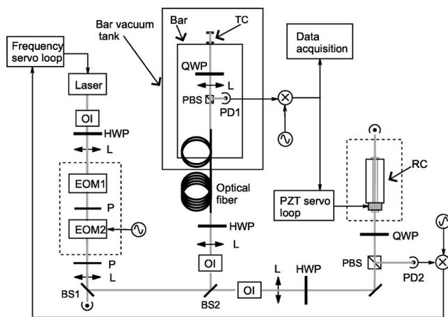
FIG. 1. Experimental setup: the drawing is not to scale. OI: optical isolator; HWP: half-wave plate; QWP: quarter-wave plate; L: lens; EOM1, EOM2: electro-optic modulators; P: polarizer; BS1, BS2: beam-splitters; PBS: polarizing beam-splitter; PD1, PD2: photodiodes; RC: reference cavity; TC: transducer cavity. Dashed lines mark out active thermal stabilization.
