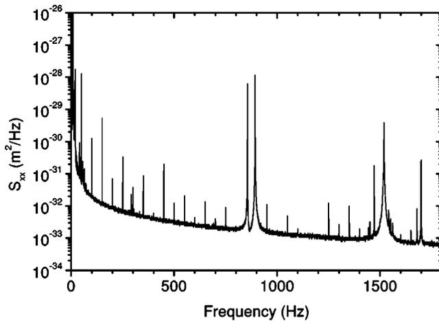
FIG. 2. Power spectral density  $S_{xx}$  of the displacement noise. The two peaks at 856 and 892 Hz correspond to the two mechanical modes of the coupled oscillators system formed by the bar first longitudinal mode and the transducer. Some other mechanical resonances are visible too. The sharp peaks at multiples of 50 Hz are due to the power line.
