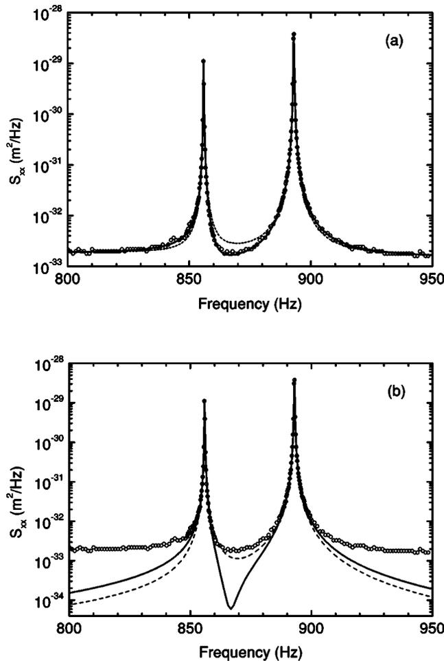
FIG. 3. (a) Power spectral density of the displacement noise. Circles: experimental data; solid line: fit according to the two-oscillators model of Eqs. (3) and (4); dashed line: fit according to the normal mode expansion. (b) The same as in (a), where the fitted curves are plotted without the wide-band  $\sim 1/f$  contribution.
