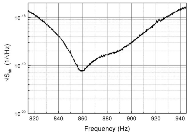
FIG. 7. Sensitivity of the GW detector, expressed in terms of the equivalent strain noise at the bar detector input. The data correspond to a 1 h average.
