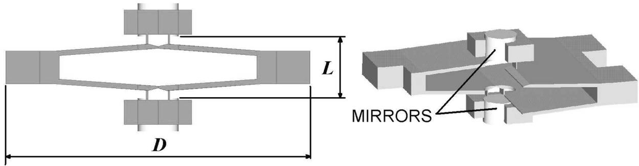
**Figure 3.** A leverage prototype: the variation on its length  $D$  represents the displacement signal and are converted in variations on the distance  $L$ . The displacement  $L$  can be measured by an optical readout, and two mirror holders are placed on to the amplifier device to make the optical cavity.
