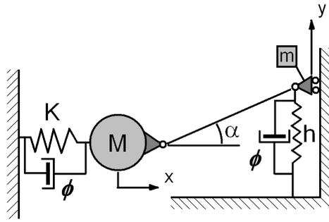
**Figure 5.** a) Lumped elements mechanical model of the amplifier+test resonator system. The mass  $M$  is the oscillators effective mass. The mass  $m$  represents the mirror+support effective mass.  $K$  is the stiffness of the oscillator and  $h$  is the amplifier one. The beam is considered rigid and of negligible mass. The same structural dissipation ( $\phi$ ) was considered for both amplifier and oscillator. b) System transfer function predicted by FEM simulation.
