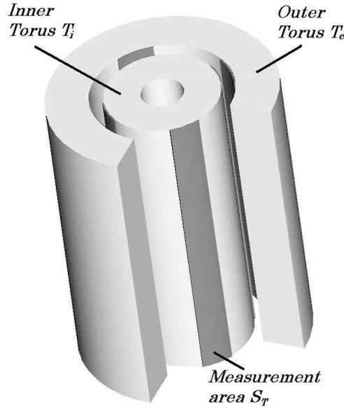
**Figure 1.** The detector is made of two concentric cylinders,  $T_e$ ,  $T_i$ . The inner cylinder may also have null internal radius. The optimally oriented gravitational wave travels along the  $z$ -axis and induces relative displacements among the two cylinders. The output signal is obtained by measuring the relative distance in 4 regions (in black), each of area  $S_r$ , for the whole cylinder height.
