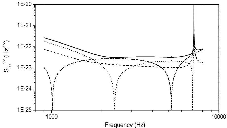
**Figure 2.** The contribution to the detector noise at the SQL is evaluated for a Molybdenum detector. Continuous line: total noise. Dashed line: thermal noise evaluated at  $T/Q \sim 2 \times 10^{-7} \text{ K}^{-1}$ . Dashed-dotted line: amplifier displacement noise. Dotted line: amplifier back-action noise.
