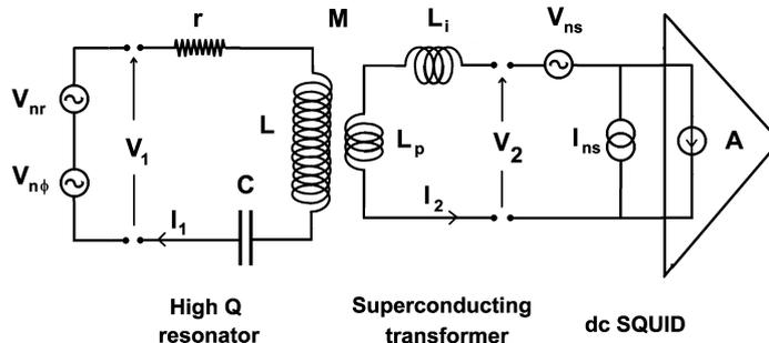
Figure 2: Schematic of the resonator with the SQUID used to measure the noise currents.
