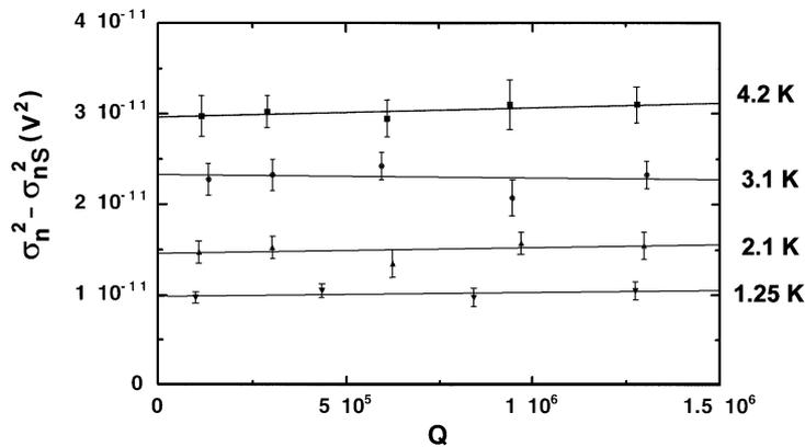
Figure 7: Variance of the SQUID output noise less the wide band SQUID noise contribution at different temperatures as a function of the quality factor  $Q$ .
