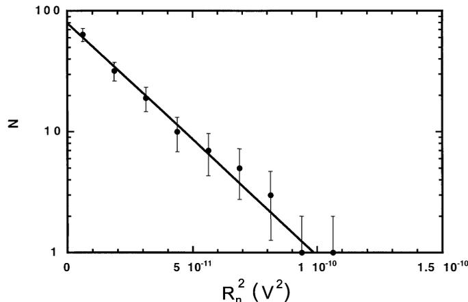
Figure 6: Histogram of the number of samples of  $R_n^2$  for each interval  $\Delta_{R_n^2} = 1.2 \times 10^{-12} \text{ V}^2$ . The solid line fits the distribution Eq. 13 with  $\sigma_n^2$  as fitting parameter.
