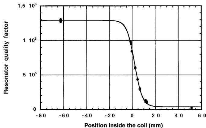
Figure 4: Resonator quality factor as a function of the position of the copper cylinder end inside the coil.
