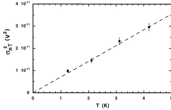
Figure 8: Thermal contribution  $\sigma_{nT}^2$  as a function of the liquid helium bath temperature. The dashed line is the theoretical expectation of Eq. 12 with no free parameters.
