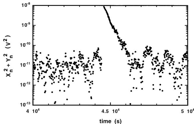
Figure 5: SQUID output squared amplitude  $R_n^2 = X_n^2 + Y_n^2$  as a function of time at  $Q \sim 10^6$ . The phases from the lock-in with  $\tau_{lk} = 3$  s were sampled at 16 s, resonator time constant is  $\tau \sim 446$  s. Unperturbed behaviour is shown together with an infrequent impulsive event, with energy more than 100 times the average one; after the sharp rising the system decays with its time constant.
