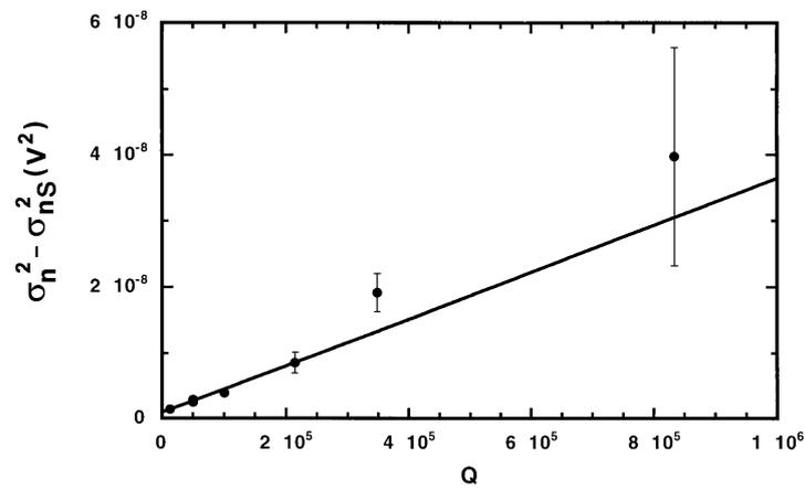
Figure 9: Variance of the SQUID output noise less the wide band SQUID noise contribution as a function of the quality factor  $Q$  in a bad shielding condition.
