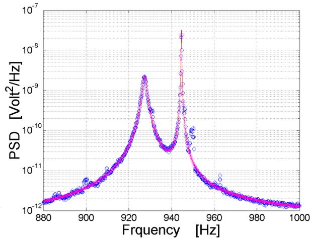
Figure 3: The measured Power Spectral Density (PSD) of the SQUID amplifier output. The fitting function (continuous line) is given in eq.1. When the readout is at liquid helium the fit estimates  $T = 4.2 \pm 0.4$  K, in agreement with the thermodynamic temperature.
