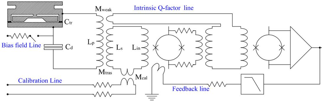
Figure 1: Scheme of the capacitive readout of the second AURIGA.
